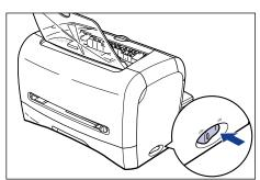
The power indicator lights up and the printer initiates a self-diagnostic test. If no abnormality is found out in the self-diagnostic test, the printer is ready to print.
