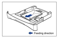
7 While holding the lock release lever on the paper guide at either side of the cassette, slide the paper guide to the mark indicating the desired envelope size.
