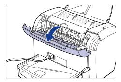
5 Tilt the two pressure release levers of the fixing unit toward you to release the pressure from the fixing unit.
