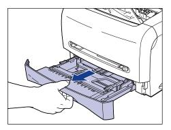
2 While holding the lock release lever on the paper guide at the rear of the cassette, slide the paper guide to the mark indicating the desired paper size.
