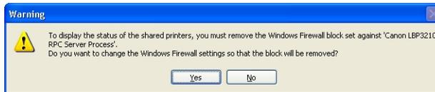
Click [Yes] to configure Windows Firewall to unblock communication with client computers. Select this option if the computer you are currently installing is a print server.
