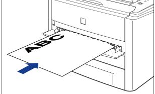
Gently insert the paper until it touches the back of the printer while supporting the paper with hands as shown in the figure.
