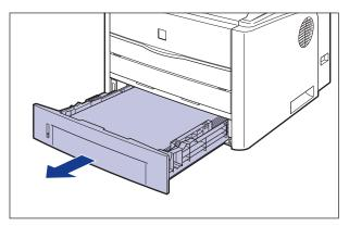
If the paper feeder is installed, pull out the paper cassette of the paper feeder also.
