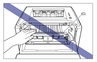
• The face-down output tray and its surroundings, and face-up output slot become hot during or immediately after using the printer. Do not touch the face-down output tray and its surroundings, and face-up output slot when removing the jammed paper or performing the related operation.
