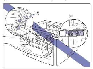
Hold the toner cartridge as shown in the figure, shake it gently 5 or 6 times to evenly distribute the toner inside the cartridge.
