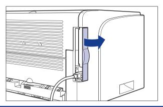
**2** Turn the printer and computer OFF ①, remove the USB cable 2, and then disconnect the power plug from the AC power outlet 3.
