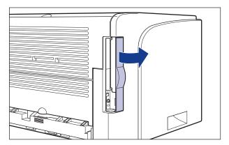
3 Connect the B-type (square) end of the USB cable to the USB connector on the rear side of the printer, then close the expansion slot cover.
