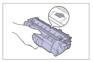
27 Push the toner cartridge into the printer until it touches the back of the printer while aligning (A) on both sides of the toner cartridge with the toner cartridge guides inside the printer.
