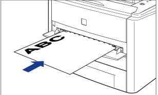
3 Gently insert the paper until it touches the back of the printer while supporting the paper with hands as shown in the figure.
