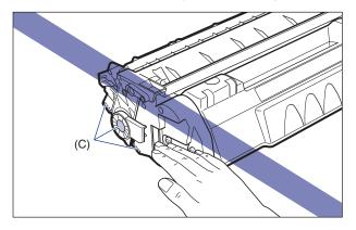
• When handling the toner cartridge, hold it properly as shown in the figure and handle it with the arrowed side facing up. Do not place it vertically or upside-down.
