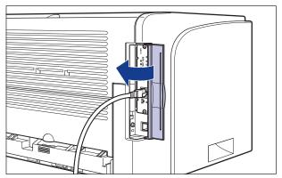
4 Connect the other end of the LAN cable to the hub.
