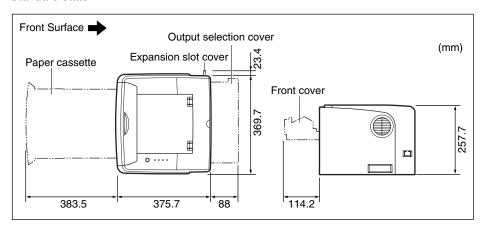
• State with the paper feeder installed
