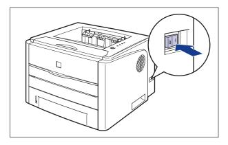
All the indicators blink, and the printer initiates a self-diagnostic test on the printer unit and optional accessories.
