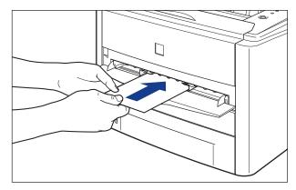
When the paper is loaded, it is sent into the slot a little.
