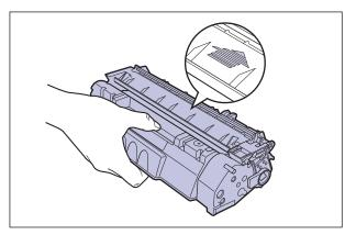
Push the toner cartridge into the printer until it touches the back of the printer while aligning (A) on both sides of the toner cartridge with the toner cartridge guides inside the printer.
