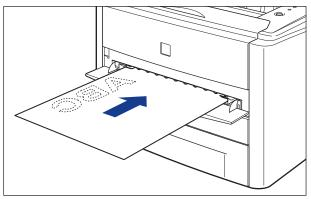
• Load paper in Cassette 2 (Only when the optional paper feeder is installed) in the same manner as you load paper in Cassette 1.
