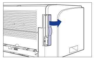
Connect the B-type (square) end of the USB cable to the USB connector on the printer, then close the expansion slot cover.
