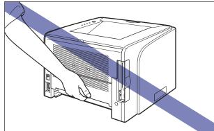
• The back portion (A) of the printer is relatively heavy. Be careful not to get off-balanced when lifting the printer. If you do so, you may drop the printer, resulting in personal injury.
