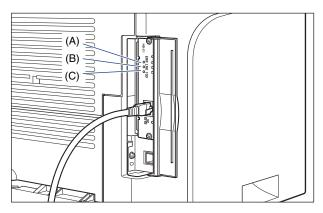
If the network board is not working properly, turn the printer OFF, and then check the LAN cable connection, hub performance, and network board installation.
