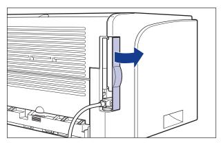
**2** Turn the printer and computer OFF ①, remove the USB cable ②, and then disconnect the power plug from the AC power outlet ③.
