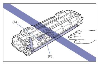
6 Hold the toner cartridge properly with the arrowed side facing up as shown in the figure.
