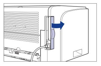
2 Turn the printer and computer OFF ①, remove the USB cable ②, and then disconnect the power plug from the AC power outlet 3.
