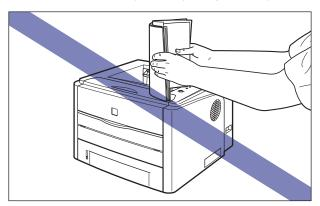
• Be sure not to open the covers on the printer during printing. This may result in damage to the printer.
