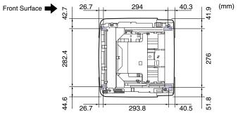
The front feet are 7.8 mm high and their top surface is 12 mm square. The rear feet are 7.8 mm high, the left top surface has a rectangular shape of 21.7 mm x 40 mm, and the right top surface is 31.7 mm x 40 mm and is L-shaped.
