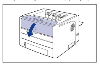
Remove the toner cartridge from the printer.
