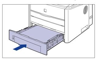
If the paper feeder is installed, set the paper cassette of the paper feeder also.
