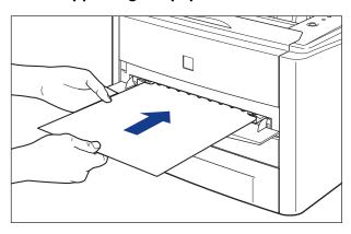
When the paper is loaded, it is sent into the slot a little.
