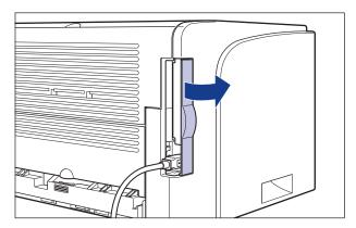
Turn the printer and computer OFF  $\odot$ , remove the USB cable ②, and then disconnect the power plug from the AC power outlet 3.
