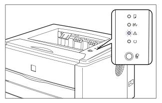
When the A (Alarm) indicator is on, a service error is occurring. In this case, see "Service Call Display," on p. 7-25.
