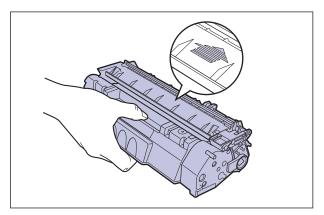
5 Push the toner cartridge into the printer until it touches the back of the printer while aligning (A) on both sides of the toner cartridge with the toner cartridge guides inside the printer.
