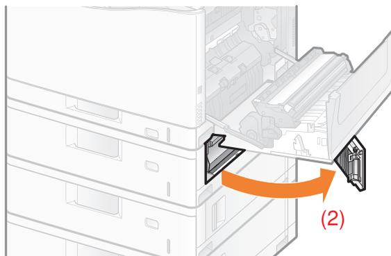
**3** Remove the jammed paper by pulling it gently in the direction of the arrow.
