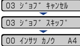
The message <03 ジョブ キャンセル> appears on the display and the print data being processed is canceled. When processing takes time, such as when receiving data, the message on the display changes to <00 ジョブ スキップ>. When the message <00 インサツ カノウ> appears on the display, job cancel is complete.
