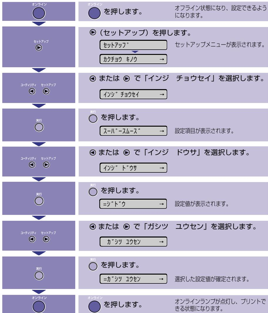
The diagram illustrates the steps to set the printer's print quality to 'Image Quality Priority' through the common setup menu. It shows the state of the printer (Online/Offline) and the menu items being navigated using the arrow keys.
