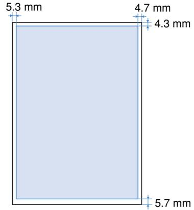
\* The printer may not be able to print correctly in areas 5 mm from the top, 10 mm from the bottom and 7.5 mm from each side.
