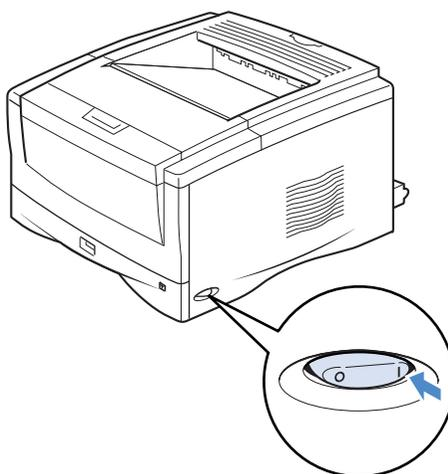
If the results of the self-diagnosis are normal, printing is enabled. The オンライン indicator, the 印刷可 indicator and the selected paper feed indicator come on and the message [00 インサツ カノウ], appears on the display.
